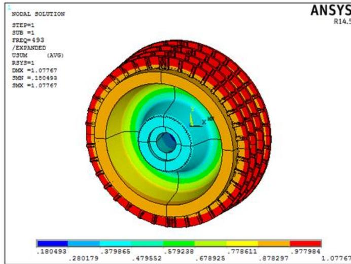
Fig 17: Mode shape corresponding to first natural frequency.
