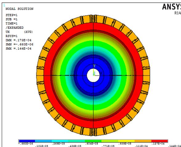
Fig 15: Radial Displacement
