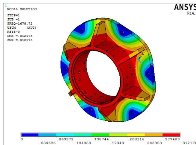
Fig 8: Mode Shape Corresponding to First Natural Frequency
