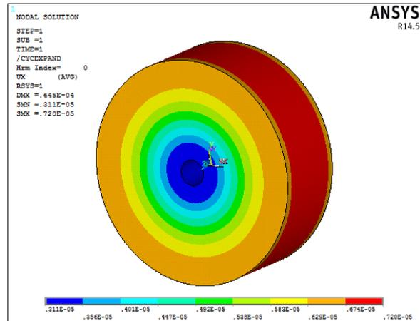
Fig 10: Radial Displacement.
