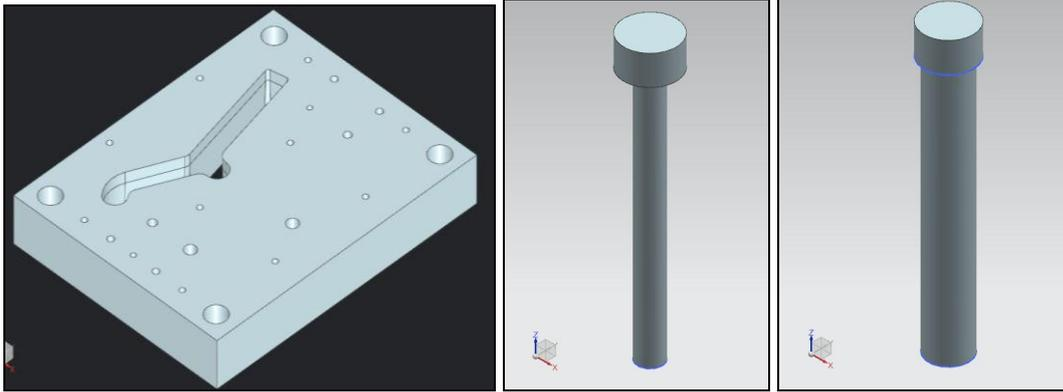
Fig 2: Progressive tool, Punch and Dies used for Blanking and Piercing operation.
