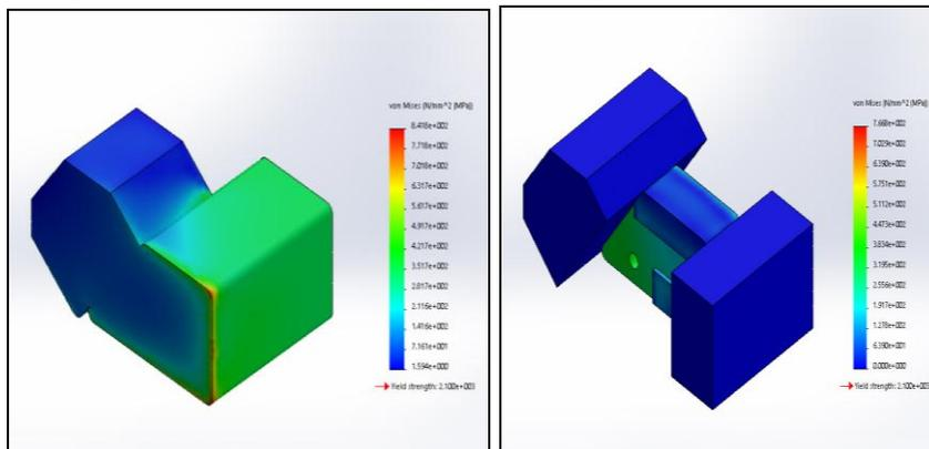
Fig 5: Maximum von-Mises Stress plots of Forming Punch and Die.
