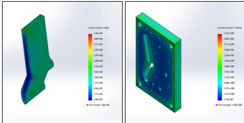
Fig 4: Maximum von-Mises Stress plots of Blanking Punch and Die.
