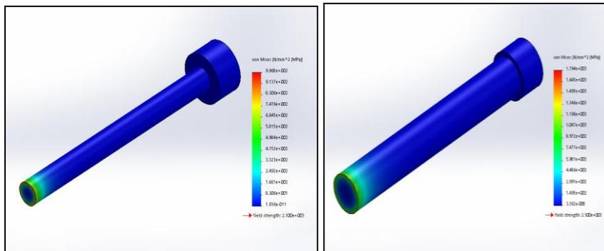
Fig 5: Maximum von-Mises Stress plots of Piercing Punch of Dia 8 and Dia 13.
