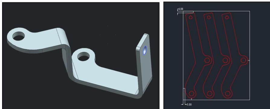
Fig 1: 3D Model of the Component and Strip Layout of the Component.
