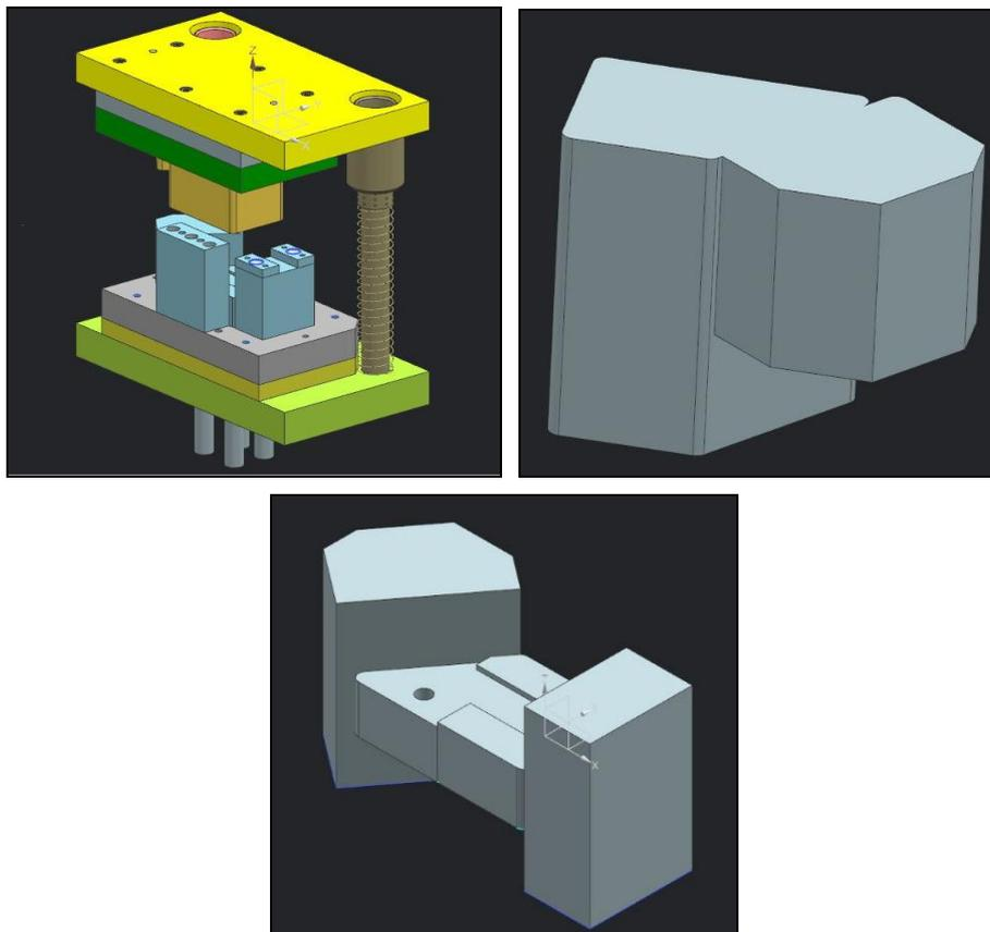
Fig 3: Forming tool, Punch and Dies used for Forming Operation.
